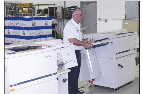
Manuel Duran works with Copresco's automated Alpha-Doc punching systems for large plastic coil bound projects.
